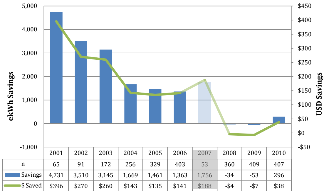
FIGURE 3: ANNUAL ENERGY AND UTILITY BILL SAVINGS ESTIMATES FOR GAINESVILLE, FLORIDA HERS-RATED HOMES.
