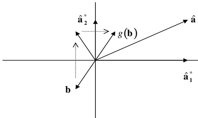
The algorithm for ML distance normalization moves  $\mathbf{b}$  along the dotted lines to element  $g(\mathbf{b})$  that has the shortest distance from  $\hat{\mathbf{a}}$ . Now, consider a general case which  $\mathbf{b}$  may not be lie completely in the span of  $\hat{\mathbf{a}}_1^*$  and  $\hat{\mathbf{a}}_2^*$ . In this case, decompose  $\mathbf{b}$  into two components: the
